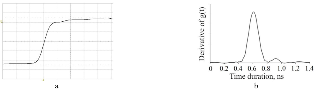
Fig. 2. The signal response oscillogram of the calibrator (rise time 25 ps) with the registering channel – a (200 ps per square (for a square)) and the derivative of this signal – b.
