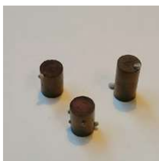
Fig. 1. Photograph of pressed Al+CuO system after sintering.
