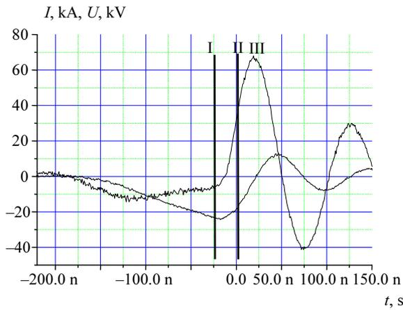
Fig. 2. Experimental temporal evolutions of capacitor  $C_2$  voltage  $U$ , current  $I$ , and lasing power ( $P$ )
