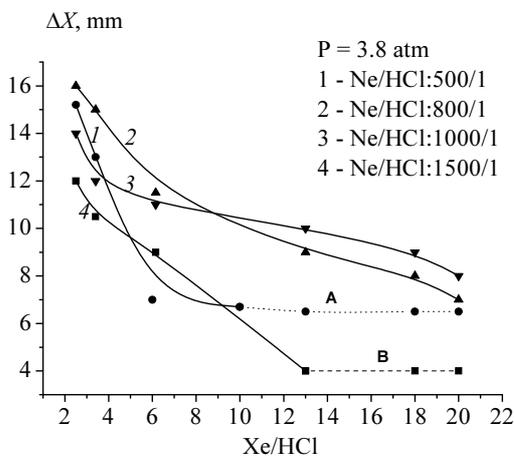
Fig. 3. Dependence of discharge width from Xe concentration
