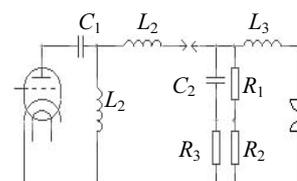
Fig. 1. Schematic diagram of excitation circuit:  $C_1 = 106.2 \text{ nF}$ ;  $C_2 = 74.8 \text{ nF}$ ;  $L_1 = 150 \text{ nH}$ ;  $L_2 = 4 \text{ nH}$ ;  $R_3$  – current shunt,  $R_1/R_2$  – resistor divider
