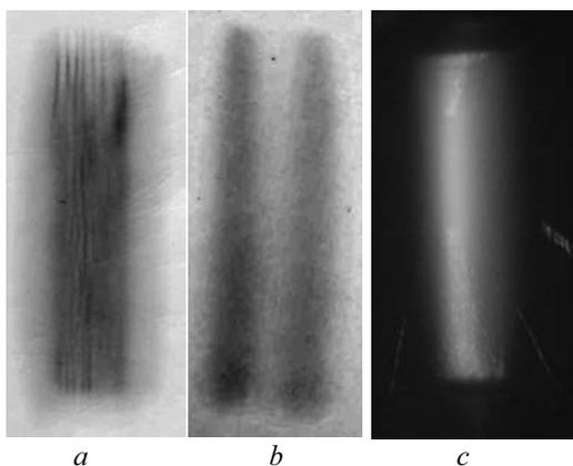
Fig. 4. laser beam autographs: *a* – Ne/Xe/HCl:500/20/1; *b* – Ne/Xe/HCl:1500/20/1 and photo the discharge; *c* – Ne/Xe/HCl:1500/20/1
