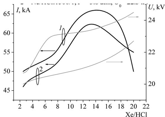
Fig. 5. Dependences of current and voltage for various concentration of halogen in the mix Ne/HCl = 500/1 (1) and 2 – Ne/HCl = 1500/1 (2) at  $P = 3.8 \text{ atm.}$ ,  $U_0 = 22.5 \text{ kV}$  for various Xe concentrations
