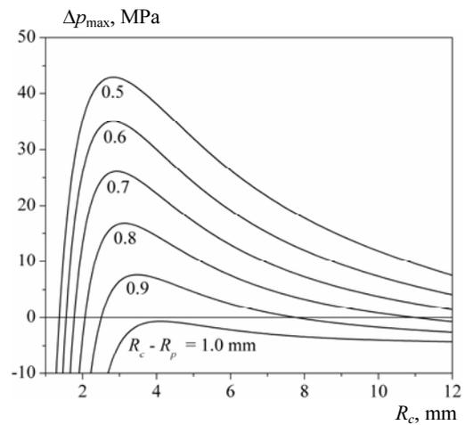
Fig. 4. Maximal value of excess pressure upon the yield point as a function of the shell outside radius  $R_c$  at the different wall thicknesses and the fixed charging voltage,  $U_0 = 13$  kV
