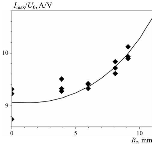
Fig. 3. Maximum value of the current passing through the solenoid as a function of the shell radius  $R_c$ . The shell thickness is 1.0 mm, the shell material is copper. Line is theoretical curve, symbols are experimental data
