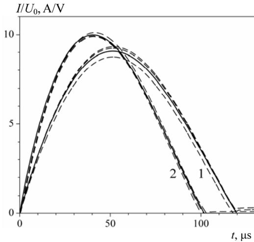
Fig. 2. Comparison between experimental and theoretical data concerning the time-dependence of the current. 1: the solenoid without shell, 2: the “solenoid + shell” system. Solid lines are theoretical ( $r_e = 6.0$  milliohm,  $l_e = 0.45 \mu\text{H}$ ). Dashed lines are experimental at different charging voltages
