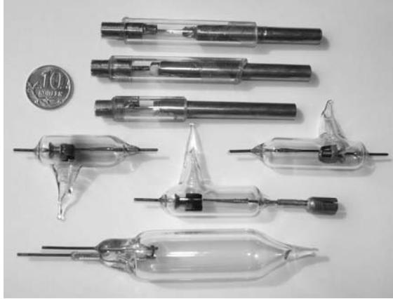
Fig. 2. Appearance of X-ray emitters with continuous evacuation and of the sealed-off type
