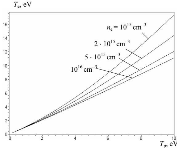
Fig. 3. Relation between  $T_p$  and  $T_e$  for different electron densities  $n_e$
