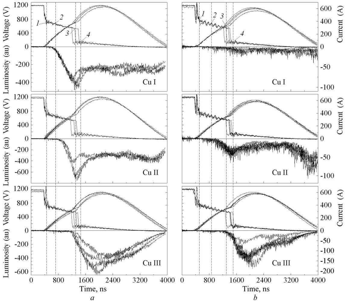
Fig. 4. Time resolved Cu lines for different discharge regions and oscillograms of the voltage and current: *a* – near the cathode edge region; *b* – discharge column. CuI,  $\lambda = 515.32$  nm; CuII,  $\lambda = 491.16$  nm; CuIII,  $\lambda = 435.19$  nm
