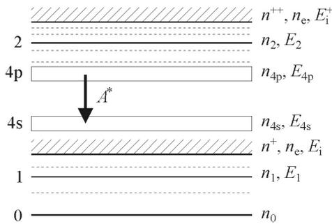
Fig. 2. Block diagram of the energy levels of CuI and CuII
