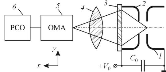
Fig. 1. Experimental setup: 1 – cathode; 2 – anode; 3 – quartz window; 4 – lens; 5 – optical multichannel analyzer; 6 – registration adaptor
