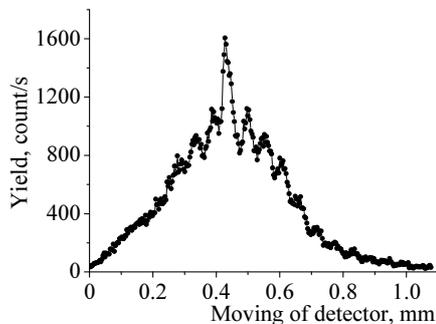
Fig. 3. Angular distribution of quantity of  $H^+$  ions transmitted through a capillary with a diameter of 0.1 mm and a length of 30 mm
