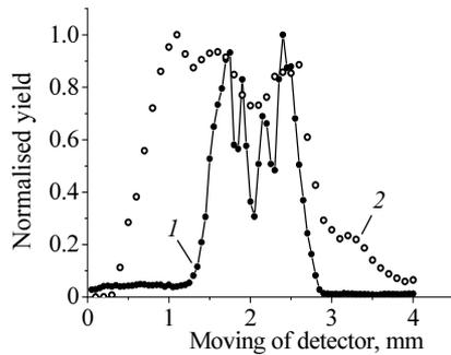
Fig. 2. Angular distribution of  $H^+$  ions ( $E = 240$  keV) transmitted through capillaries with a diameter of 0.5 and length of (1) 178 and (2) 65 mm. The angle between the beam and the capillaries is  $0.0^\circ$
