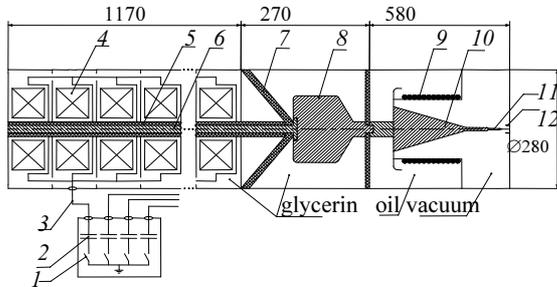
Fig.1. Electric field strength at different generator elements: 1 – HCEIcap50-0.1 capacitor ( $E = 200$  kV/mm, DC voltage); 2 – high voltage pulsed oil-filled cables ( $E = 21$  kV/mm, pulse 200 ns); 3 – insulation of the secondary winding ( $E = 100$  kV/mm, pulse 200 ns); 4 – capacitor with glycerin insulation ( $E = 21$  kV/mm, pulse 200 ns); 5 – surface strength in vacuum ( $E = 3$  kV/mm, pulse 200 ns)
