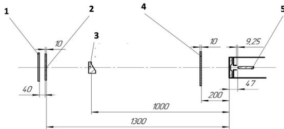
Fig. 4. Arrangement of the test objects: 1 – photoplate (x-ray plate); 2 – duralumin plate; 3 – object; 4 – glass textolite; 5 – anode
