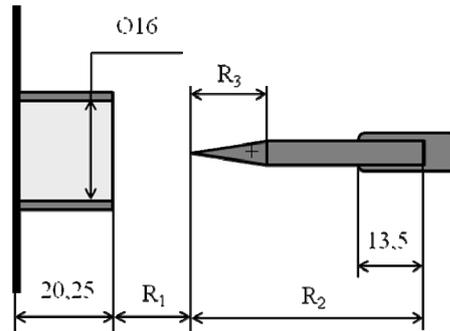
Fig. 2. Design of the cathode-anode unit.  $R_1 = 9.25$  mm,  $R_2 = 47$  mm,  $R_3 = 5.5$  mm
