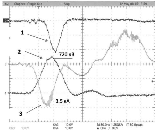
Fig. 3. Oscillograms: 1 – signal from SKD1-0.1; 2 – load voltage; 3 – load current
