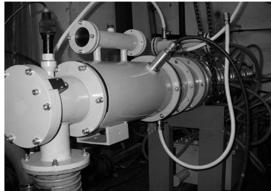
Fig. 6. Photo of the x-ray source
