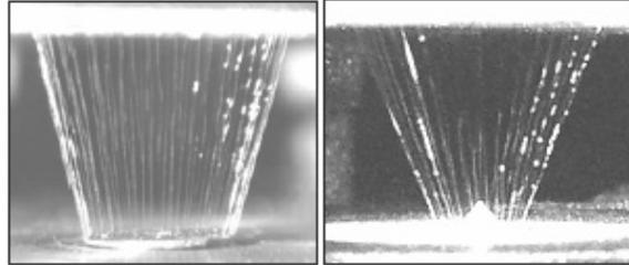
Fig. 1. Conical wire arrays with flat and cone-shaped cathodes
