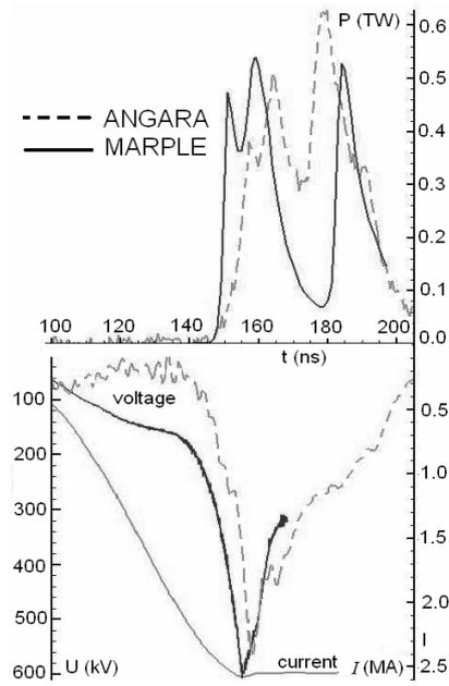
Fig. 2. Voltage (kV) and SXR-pulse (TW) (ANGARA – experiment, MARPLE – simulation)
