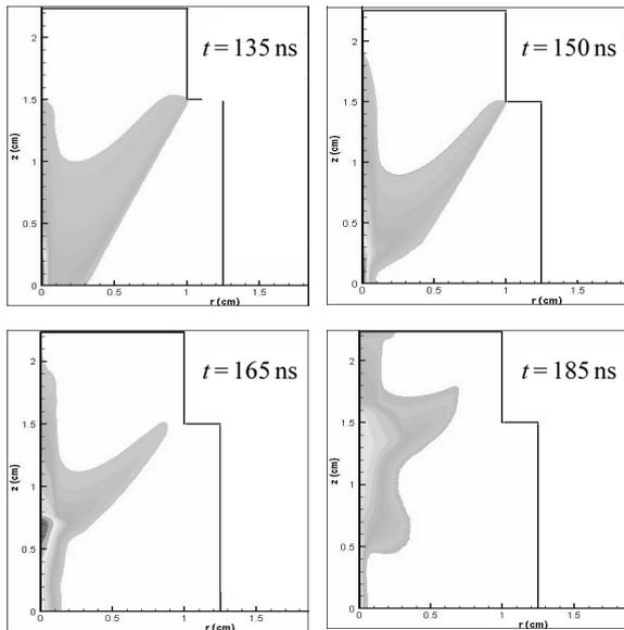
Fig. 3. Pinch shape in 4482 simulation ( $t = 135$  ns – precursor formation;  $t = 150$  ns – SXR prepulse;  $t = 165$  ns – the first SXR pulse,  $t = 185$  ns – the second SXR pulse, radiating zone split)
