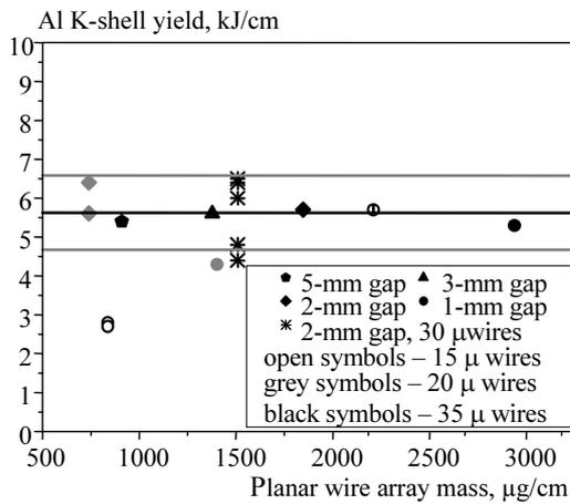
Fig. 1. Al K-shell radiation yield as a function of the planar wire array mass for 1050-ns implosions
