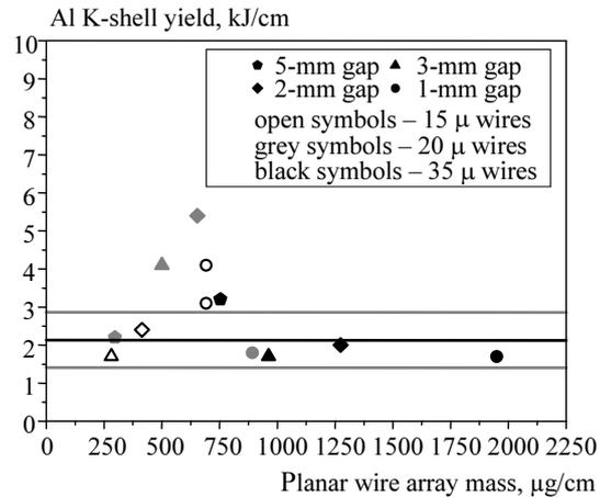
Fig. 250. Al K-shell radiation yield as a function of the planar wire array mass for 850-ns implosions.
