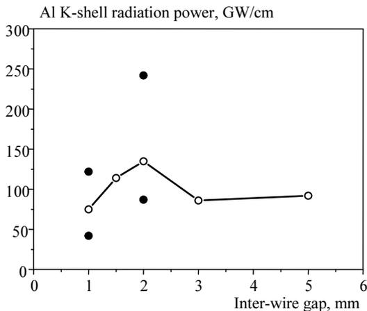
Fig. 3. Al K-shell radiation power as a function of the inter-wire gap for 1050-ns implosions
