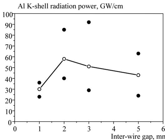
Fig. 4. Al K-shell radiation power as a function of the inter-wire gap for 850-ns implosions
