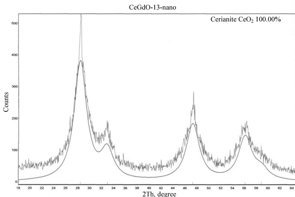
Fig. 5. Diffraction pattern of the target ( $Ce_{1-x}Gd_xO_{1-\delta}$ )
