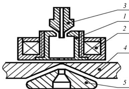
Fig. 2. Gas-discharge system of the electron source: 1 – hollow cathode; 2 – magnet; 3 – ignitor electrode; 4 – anode; 5 – accelerating electrode
