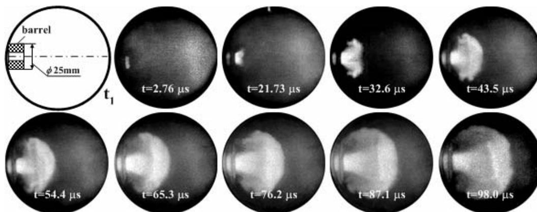
Fig. 1. Photogram of a supersonic plasma jet flowing from the acceleration channel of the titanium barrel. Experimental conditions:  $C = 48 \cdot 10^{-3}$  F,  $U_{ch} = 3.0$  kV,  $W = 113$  kJ,  $P = 1.0$  atm;  $t_1$  is the moment when plasma is coming out of the AC
