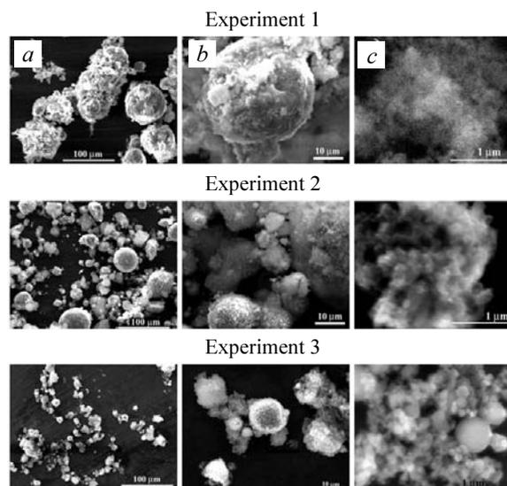
Fig. 3. Microphotographs of the dynamic synthesis powder-like products in the experiments 1, 2, and 3, Table; at different zooms
