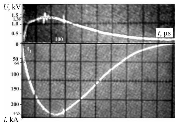
Fig. 2. Typical oscillograms of voltage on the electrodes  $u(t)$  and operating current  $i(t)$ . Experimental conditions:  $C = 48 \cdot 10^{-3}$  F,  $U_{ch} = 3.0$  kV,  $W = 113$  kJ,  $P = 1.0$  atm
