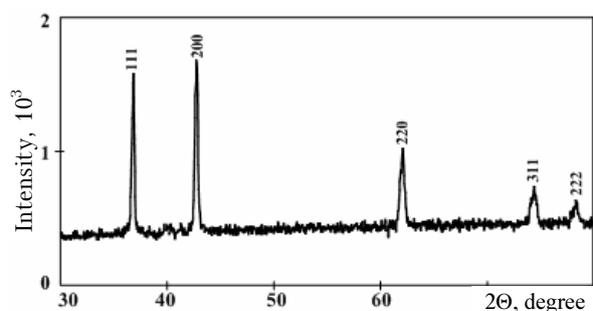
Fig. 4. X-ray diffraction pattern of the nanodispersed TiN powder with face-centered cubic arrangement
