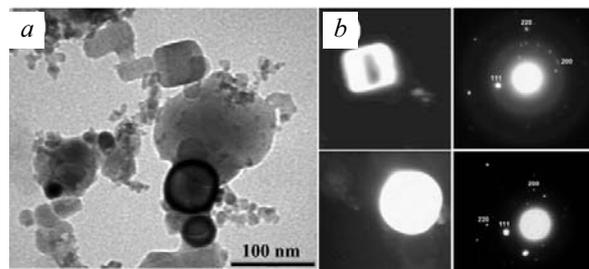
Fig. 5. Electronic microphotograph of nanodispersed powder (bright-field image) (a) and dark-field image of individual crystals with the corresponding electron diffraction patterns (b)
