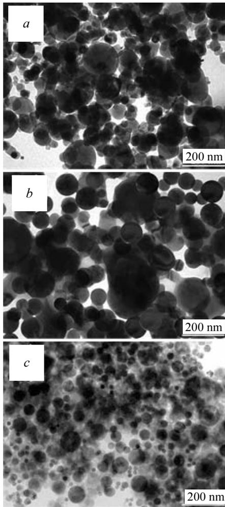
Fig. 6. Electronic microphotographs of nanodispersed powders obtained in the experiments 1 (a), 3 (b), and 4 (c), Table
