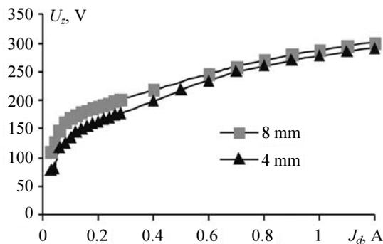
Fig. 3. The dependence of probe potential on discharge current at various distances from the target surface
