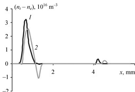
Fig. 2. The spacious distribution of excess charge for various voltages at magnetron: 1 – 225; 2 – 195 V
