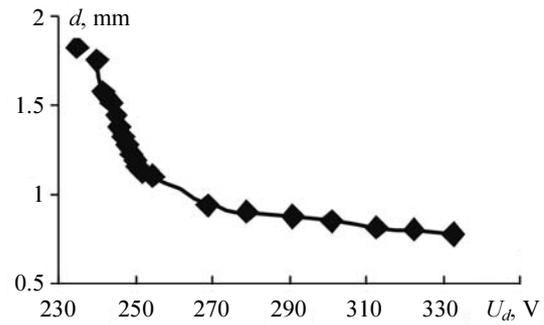
Fig. 4. The dependence of independent discharge zone size on the voltage of magnetron
