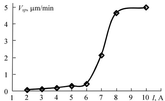
Fig. 5. The dependence of film growth speed on discharge current for copper target
