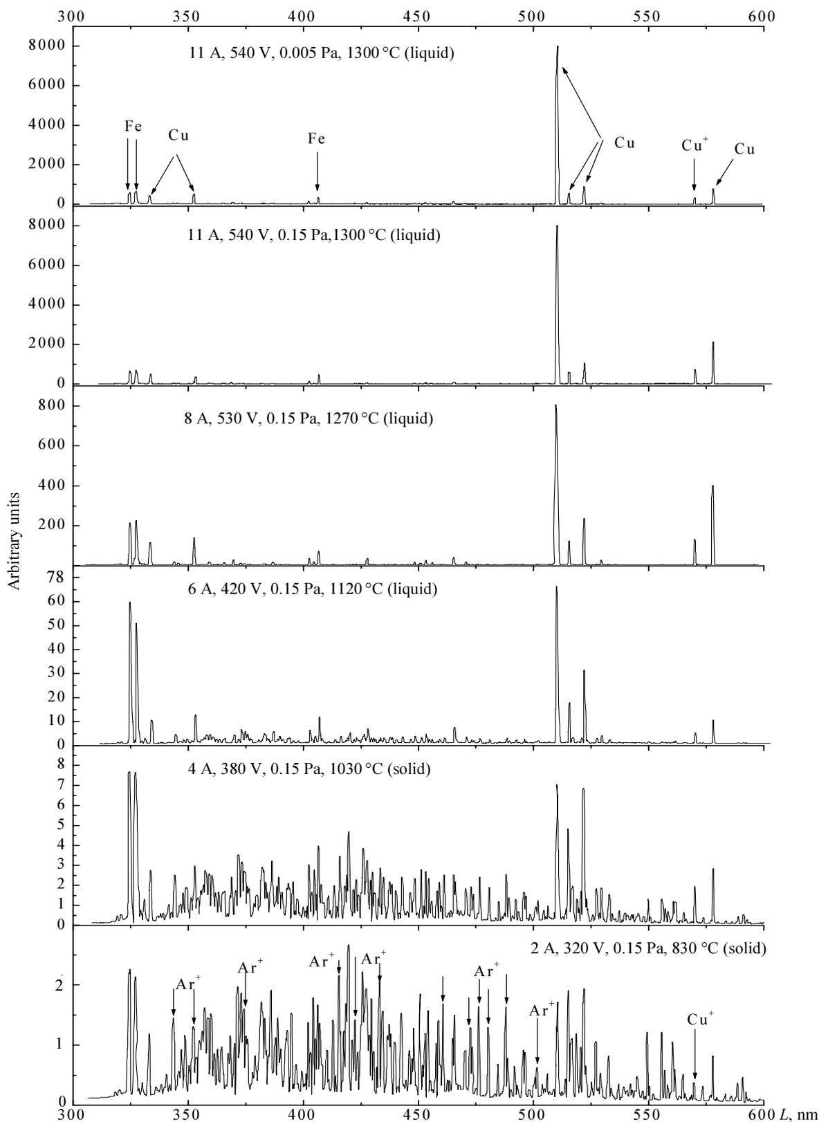
Fig. 6. Optical spectrum of the magnetron discharge plasma
