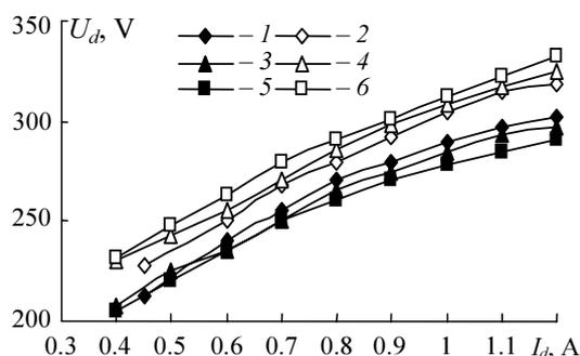
Fig. 1. The volt-ampere characteristics of magnetron (curves 1–3) and probe potential relative to cathode (curves 4–6) at various distances from the target surface: 1 and 4 – 14; 2 and 5 – 6; 3 and 6 – 4 mm
