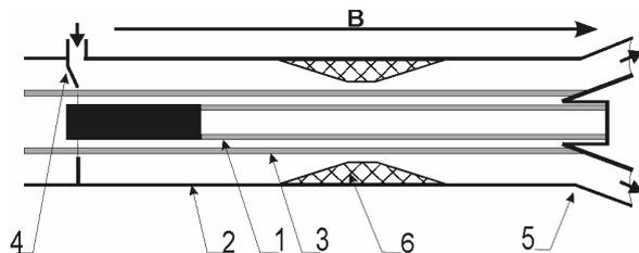
Fig.2 Experimental device. 1.- plasma, 2.-metall waveguide, 3.-electron beam, 4.- microwave power input, 5.-output microwave horn, 6.-absorber.
