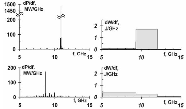
Fig.5. Frequency spectrum of microwave pulse power and energy, up -  $B = 8$  kG  $\pm 9\%$ , down -  $B = 16$  kG  $\pm 9\%$ , (computer simulation).
