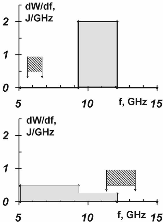
Fig.4. Frequency spectrum of microwave pulse energy, up -  $B = 8$  kG  $\pm 9\%$ , down -  $B = 16$  kG  $\pm 9\%$
