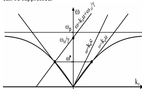
Fig1. Dispersion curves of the forward and backward plasma waves and of the space charge waves of an electron beam.
