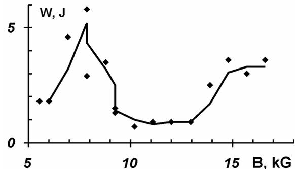
Fig.3. Microwave pulse energy on magnetic field.
