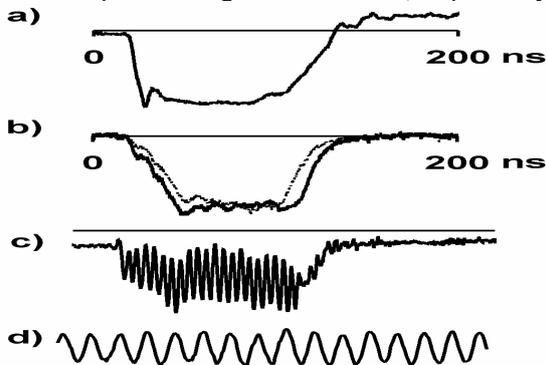
Fig.6. Typical oscillograms. a) accelerator cathode voltage, b) microwave pulses, c) beating signal, d) fragment of the same signal c) during 70 ns.
