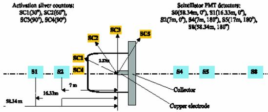
Fig.1. Location of the neutron detectors
