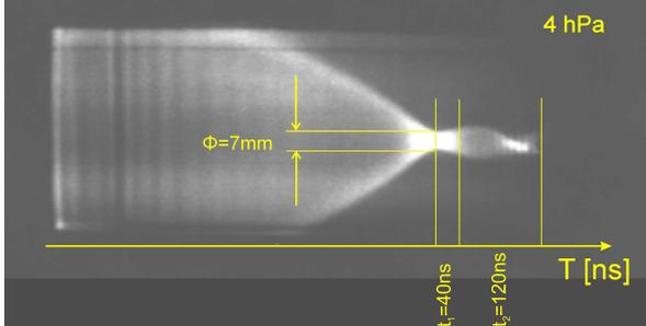
Fig.4. High-speed smear picture showing the formation of the second pinch (shot #5055)
