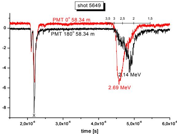
Fig.5. X-ray and fusion-neutron signals recorded at the same distance but at different angles to the z-axis
