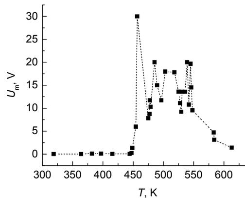
Fig. 3. Maximum Barkhausen's electric pulse height versus temperature for polarized by electric field ferrite specimens
