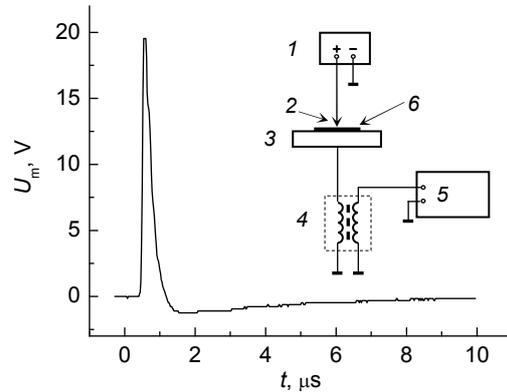
Fig. 2. Typical electric pulse form at  $T = 510$  K,  $E_p = 125$  V/cm. The insert shows the experimental schematics: direct current power supply – 1, upper electrode – 2, lower electrode with heater – 3, transformer – 4, Velleman oscilloscope – 5, and tested specimen – 6
