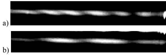
Fig. 3. Effect of frequency doubling spatial modulation of luminescence intensity of F_3^+ (a) – centers, in comparison with luminescence intensity of F_2^+ ; (b) – centers
