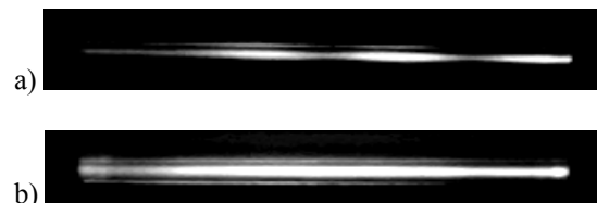
Fig. 2. Spatial distribution of luminescence intensity F_2^- (a) and F_3^+ (b) – centers in LiF crystals with induced anisotropy. Exciting light was directed into normal to plane (100)
