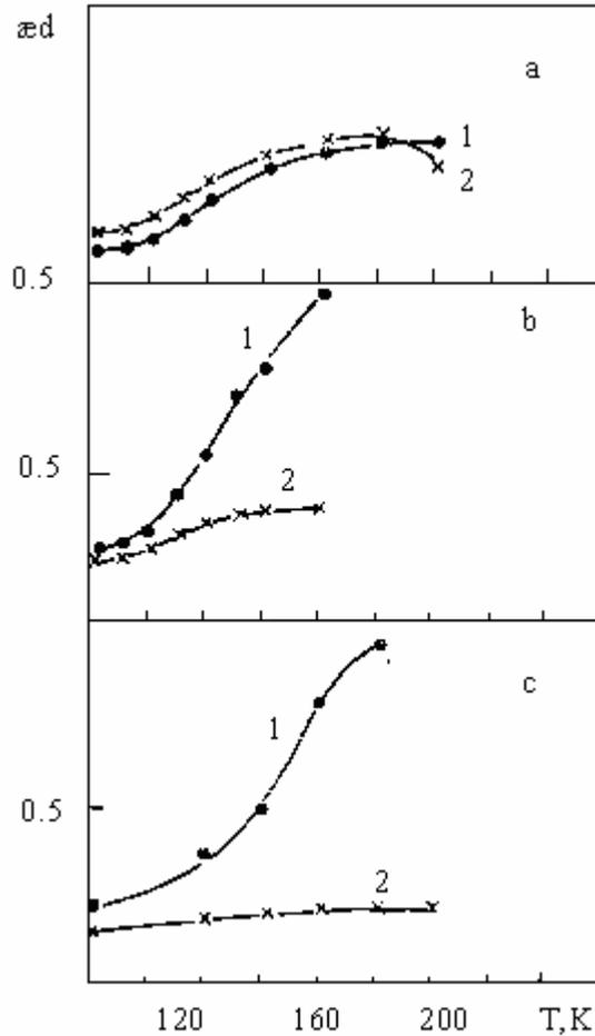
Fig. 3. Temperature dependence of the absorption in  $\alpha$  and F-bands (curves 1 and 2) in KBr-Li with concentration of Li 0.2(a), 0.004(b) and 0.0005(c) mol.%. The X-radiation times were the following: 2 min.(a), 5 min.(b) and 15 min. (c)
