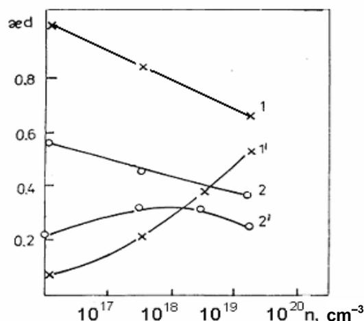
Fig. 1. Dependence of the absorption in I- band at 5.2 eV and in K-band at 2.35 eV on  $Li^+$  concentration for KBr-Li : radiated during 225 minutes for 5 K (1 and 2) and for 80 K (1' and 2')
